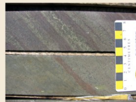
High-grade banded Zn-Pb-Cu sulphides (Boomerang Deposit).
