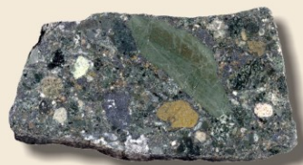
Zn-Pb-Cu breccia (transported) ore with clasts of massive sulphides (Buchans Mine).
