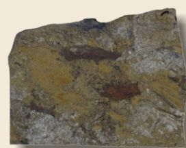
Zn-Cu-Pb-pyrite breccia ore (Duck Pond Mine).
