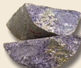
Zn-Pb-Cu massive sulphides (Lemarchant)
